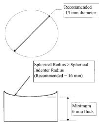
FIG. 3 Recommended Spacer Drawing
