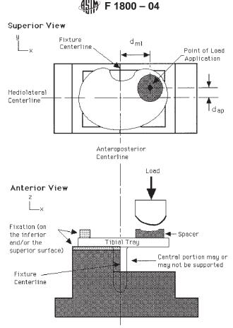
FIG. 2 Schematic or Test Setup With a Central Keel
